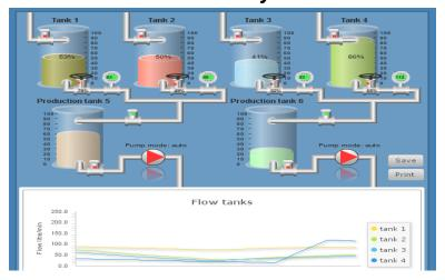
SCADA (Supervisory Control And Data Acquisition) for monitoring and control of station pumps, tanks and valves over WinCC Siemens subsystem:
